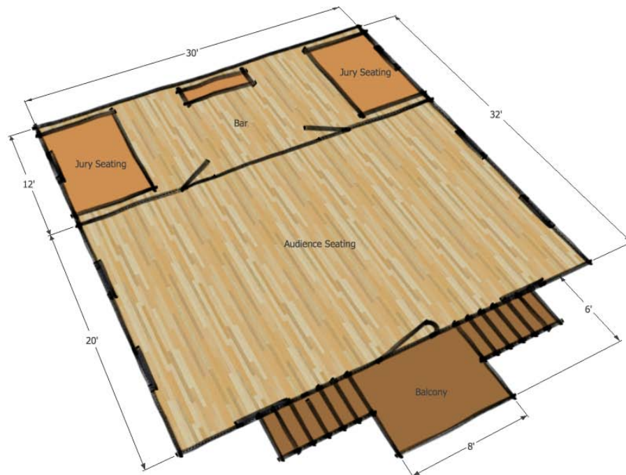
Figure 4.7. Drawing of the second floor of the 1876 Pine Level courthouse. (Drawing by the author)
